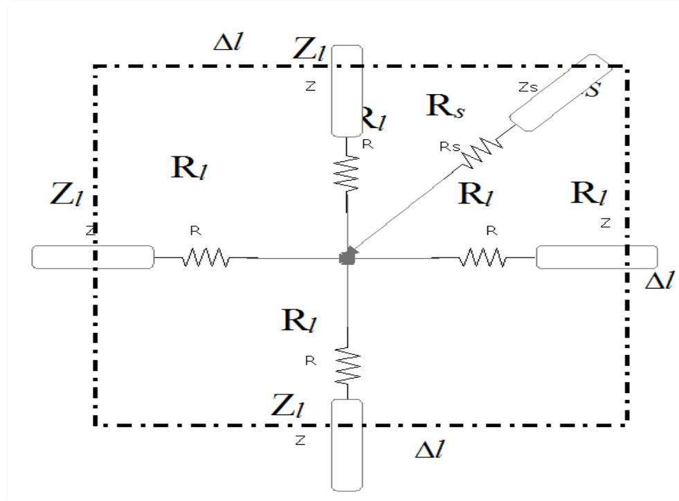
Figure-1: A TLM network with stub loaded that all the  $R_L$ s and  $Z_L$ s in the node are the same value for square element.
