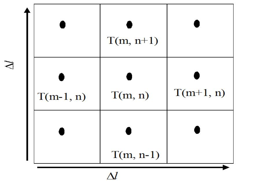
Figure-3: Spatial Relationship of Temperature represented to discretisation of parabolic heat propagation.
