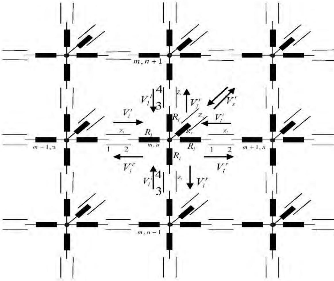
Figure-2: TLM Pulse Scattering in a 2-D node.
